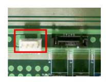
PS8P1:8-Pin Power Connector (Xeon-8P Male )
